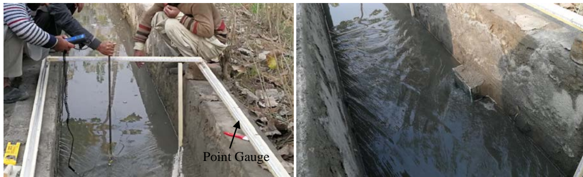
Figure 09: Model Channel, Discharge Confirmation, Abutment Set-out and flow of water in Model Channel
